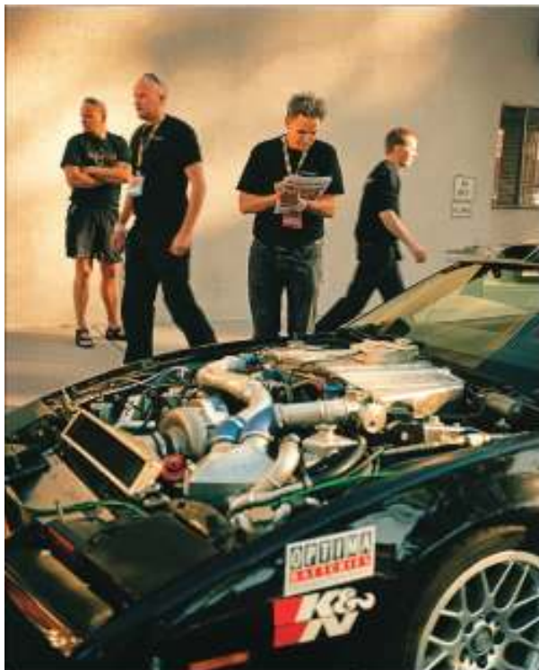
EVIL FORCES: There is not much space for more stuff under the hood. But a 8.9 litres V8, with a supercharger that develops 1407bhp might be enough. From left, not counting the tourist in the background is Gunnar Skjerve, Pal-Arvid Blytt and Arne Christian Kaland.
